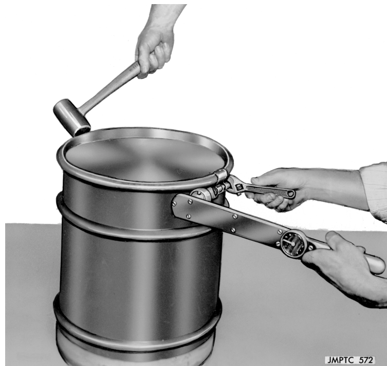
Figure 5-7. Tapping locking ring while tightening bolt to insure an effective seal (MIL-D-6054).
