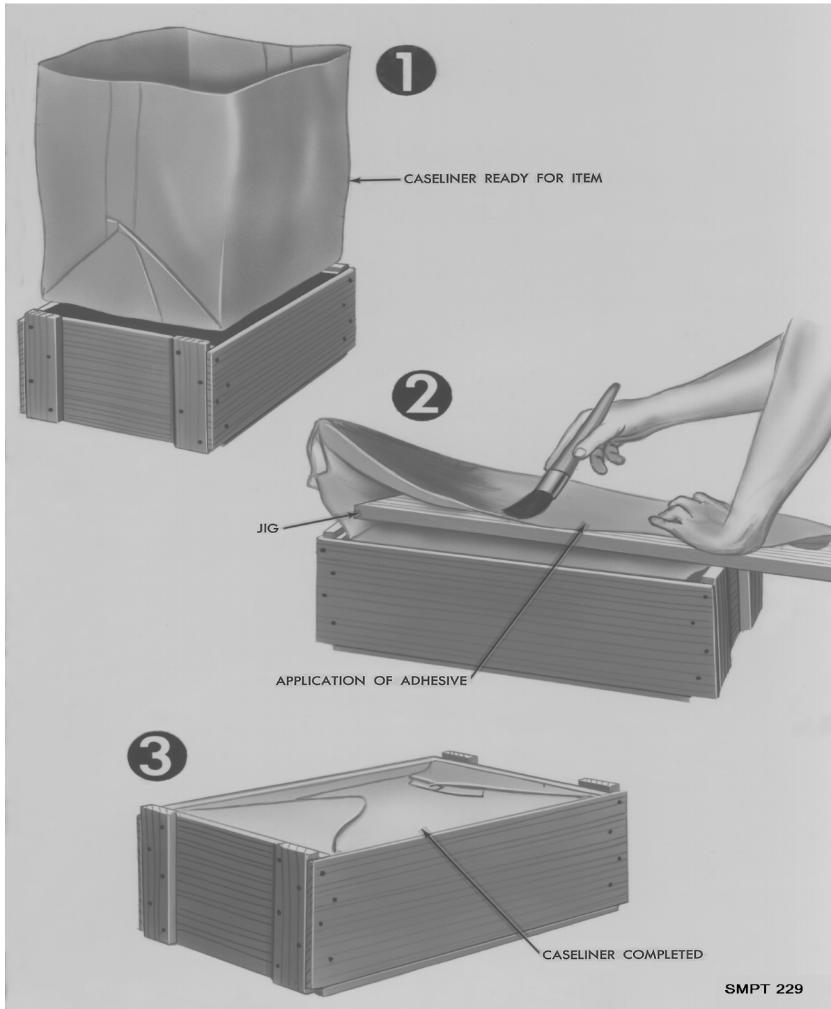
Figure 1-32. Using and closing of high top caseliner.
